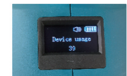
OLED display (Cutting time, Electricity QTY, Maintenance reminding and fault code)
