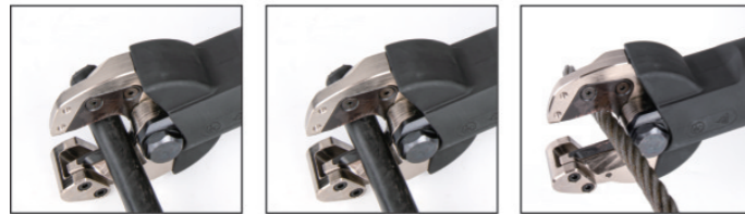
Cu/Al cable \leq\phi 26mm
